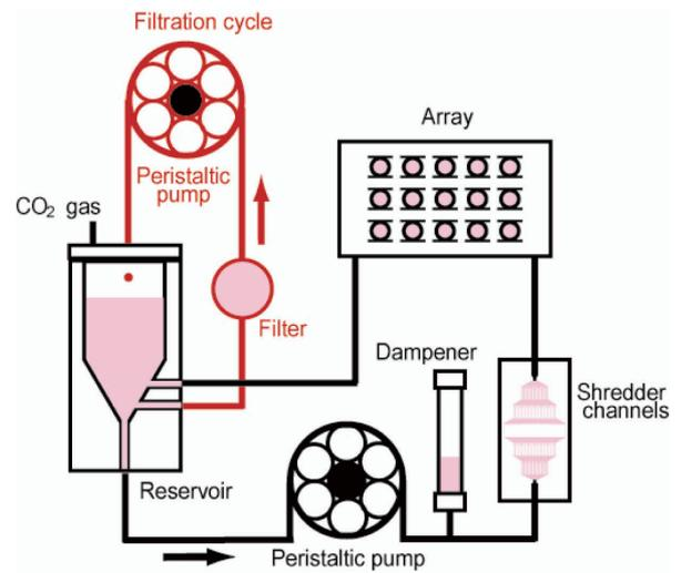
Fig. 4. Spheroid formation device consisting of an array and perfusion with a reservoir, a shredder channel, dampener, filtration cycle, and peristaltic pump.
