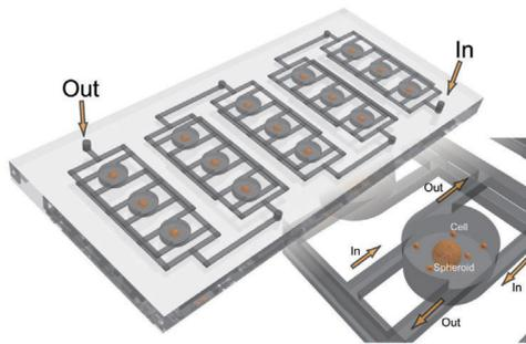
**Fig. 1.** Spheroid formation array. Hepatocytes are assembled by microrotation flow and form a spheroid in the chamber center.
