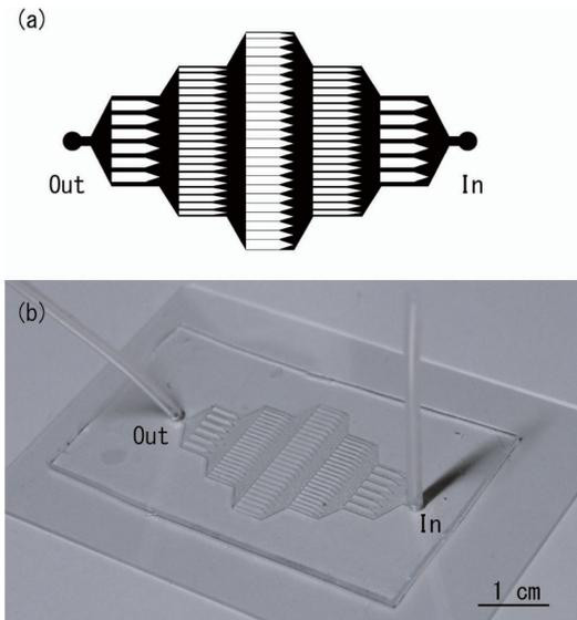
**Fig. 6.** (a) Shredder channel design. The narrowest channel was  $50\ \mu\text{m}$  in the middle. Large aggregations of cells are broken up by shear stress and/or trapped in the channel when aggregations of cells flow in the channel. (b) Shredder channel fabricated photolithographically.
