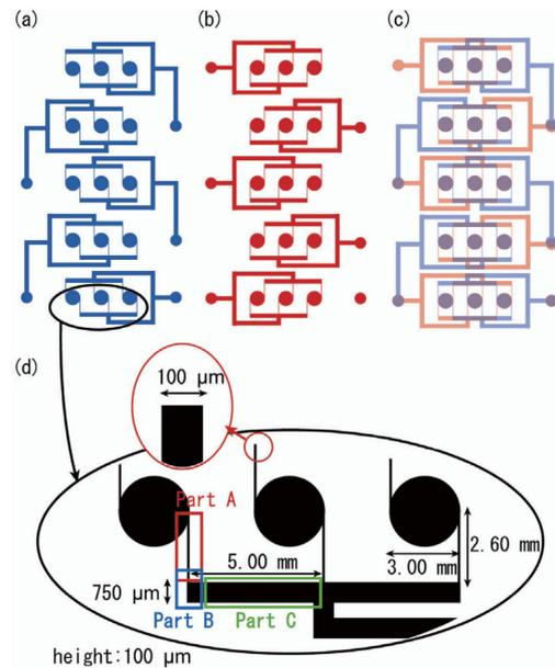
**Fig. 2.** (a) Middle and (b) upper array design. (c) Flow channel connection. (d) Magnified view of array.
