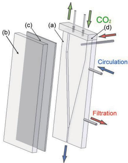
**Fig. 5.** The reservoir consisted of (a) a channel, (b) cover, (c) silicon sheet, and (d) top cover. The silicon sheet increased adhesion between (a) and (b).
