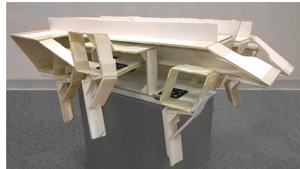
Fig. 10 A meter long hexapedal SCM robot made in the BIRDS lab at the University of Michigan. Developed by Devin Miller, Ian Fitzner, and Shai Revzen, with thanks to Stacie Desousa.
