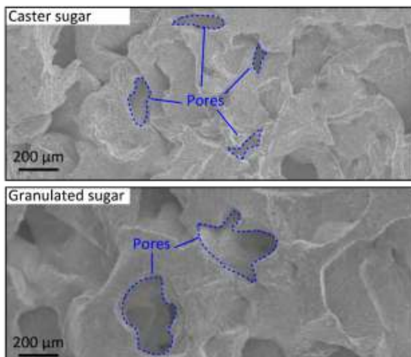
Supplementary Figure S6. Differences in pore size of caster and granulated sugar based on scanning electron microscopy images.
