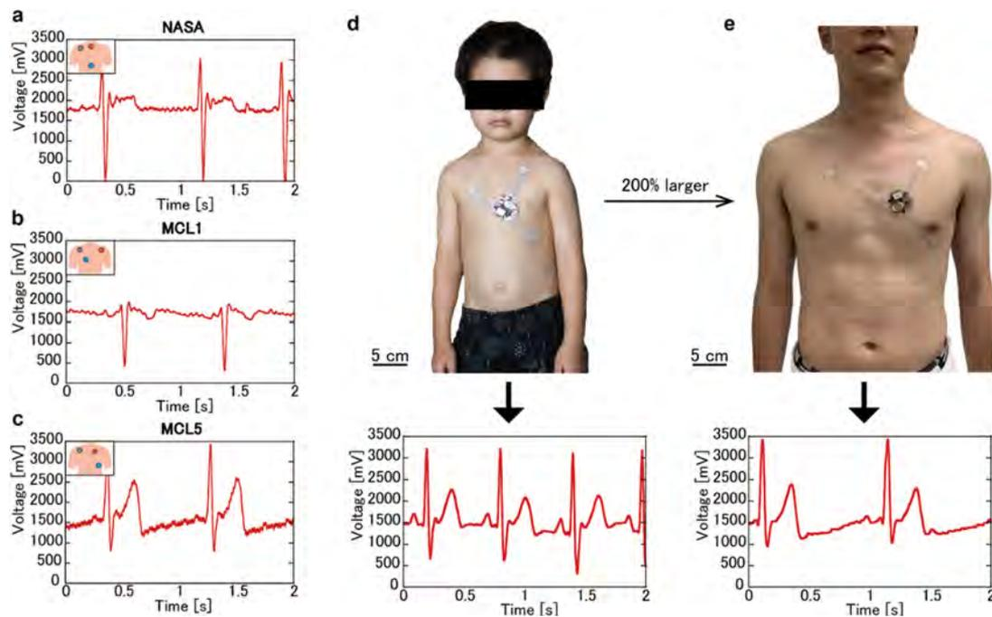
**Figure 4.** ECG measured by the developed device. (a–c) ECGs measured in NASA (a), MCL1 (b), and MCL5 (c) leads using one device. Each ECG in a different lead can be detected by the same device. (d) The device can detect the ECG for a 6-year-old child. (e) Further, the developed device can measure ECG of an adult whose chest size is two times larger than that of the child by stretching the electrodes.
