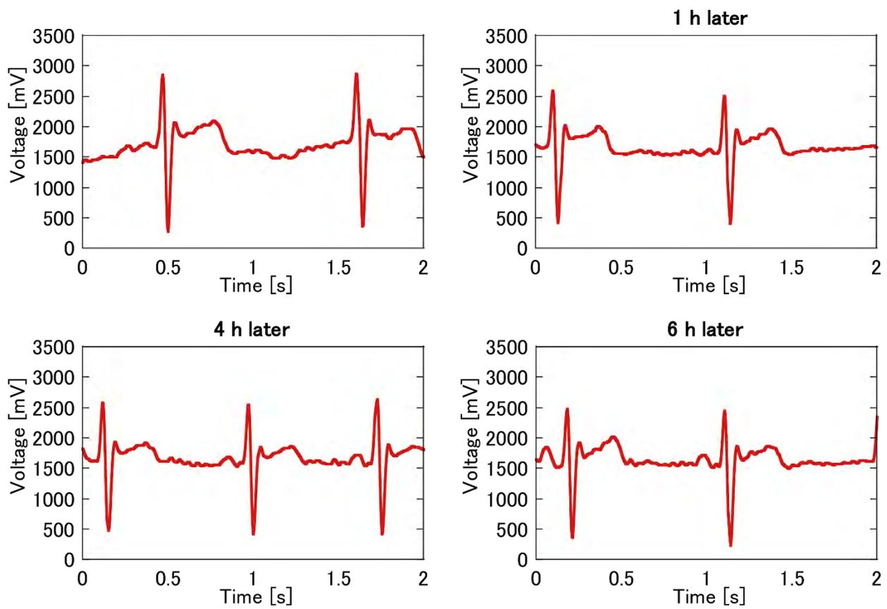
Figure S10. Long-term ECG measurement of the developed device with NASA lead (up to 6 h).
