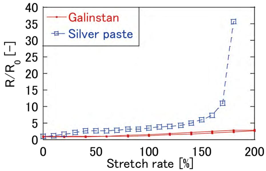
Figure S4. 200% tensile tests using silver paste and Galinstan on a stretchable substrate.
