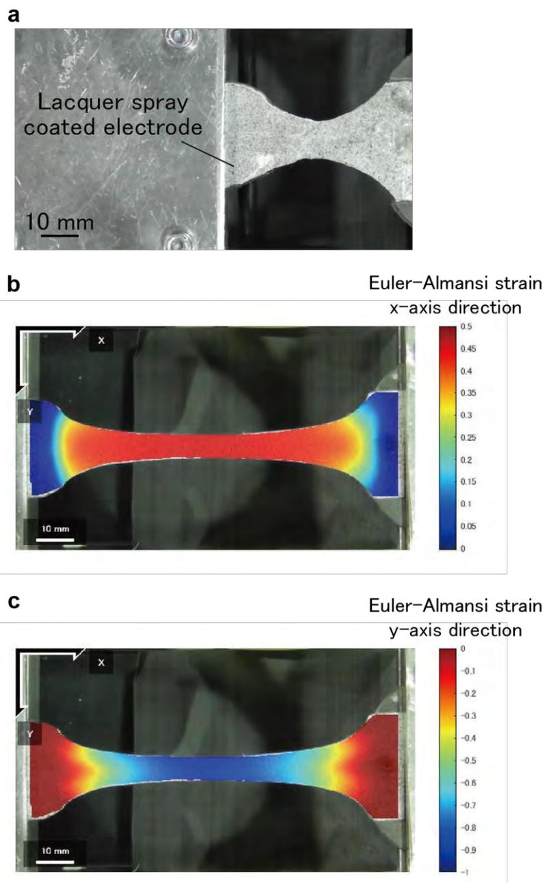
Figure S2. Strain distribution after image processing when the electrode was stretched to 200%. (a) Photograph in strain experimental condition. (b) Distribution of x-axis Euler–Almansi strain at 200% stretching. (c) Distribution of y-axis Euler–Almansi strain at 200% stretching.
