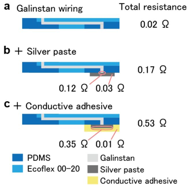
Figure S3. Breakdown of the resistance values of the stretchable electrode. The resistance values of liquid metal only, silver paste coating, and the conductive adhesive attached, and the contact resistance between liquid metal and silver paste and between the silver paste and conductive adhesive.
