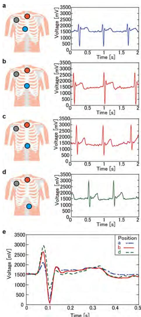
**Figure 5.** Changes in ECG based on the electrode location. (a–d) ECGs were measured in different locations of the negative electrode. The shape of the ECG was different based on the distance between the negative, positive, and ground electrodes. (e) The result of the multiple ECG signals measured in different measurement positions.
