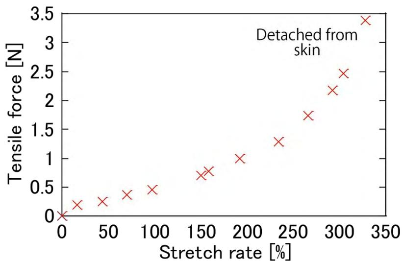
Figure S7. Evaluation of the adhesive strength of the conductive gel adhesive. Even if the electrode was stretched to 200%, the conductive adhesive did not peel off from the body surface. The tensile force when the electrode was stretched increased with strain.
