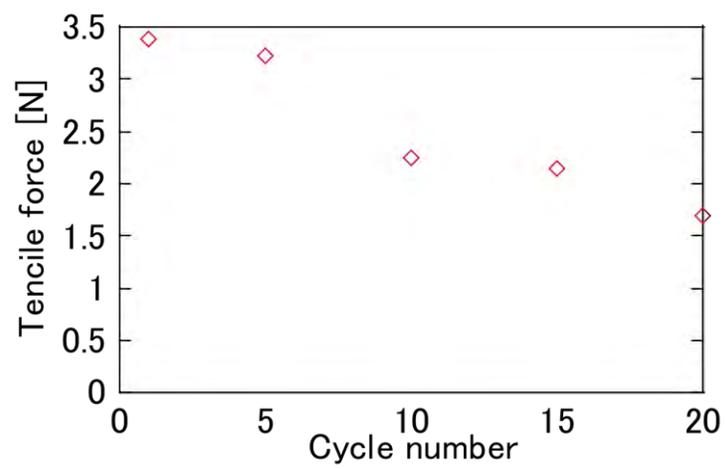
Figure S9. Reduction in the adhesive strength of conductive adhesive with respect to the number of cycles
